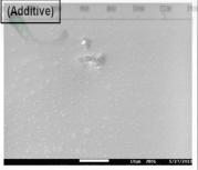
Metal surface image under at 150 °C, 50 bar pressure in 2 wt% NH<sub>4</sub>C
