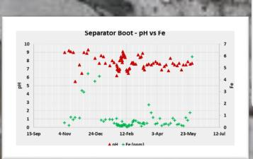
Field Trial results in NHT-ISOM-Separator outlet boot water
