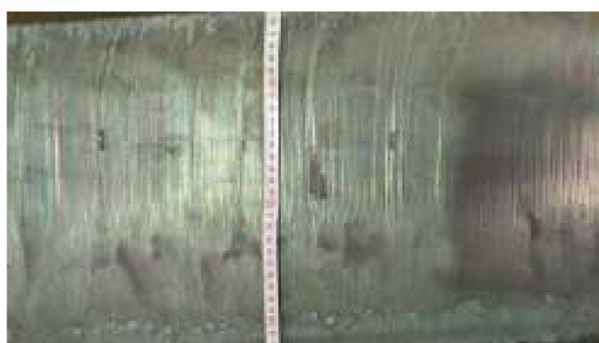
Fig. 15. Smooth Cut Surface Profile 300 mm (Close up View) using RAZOR
