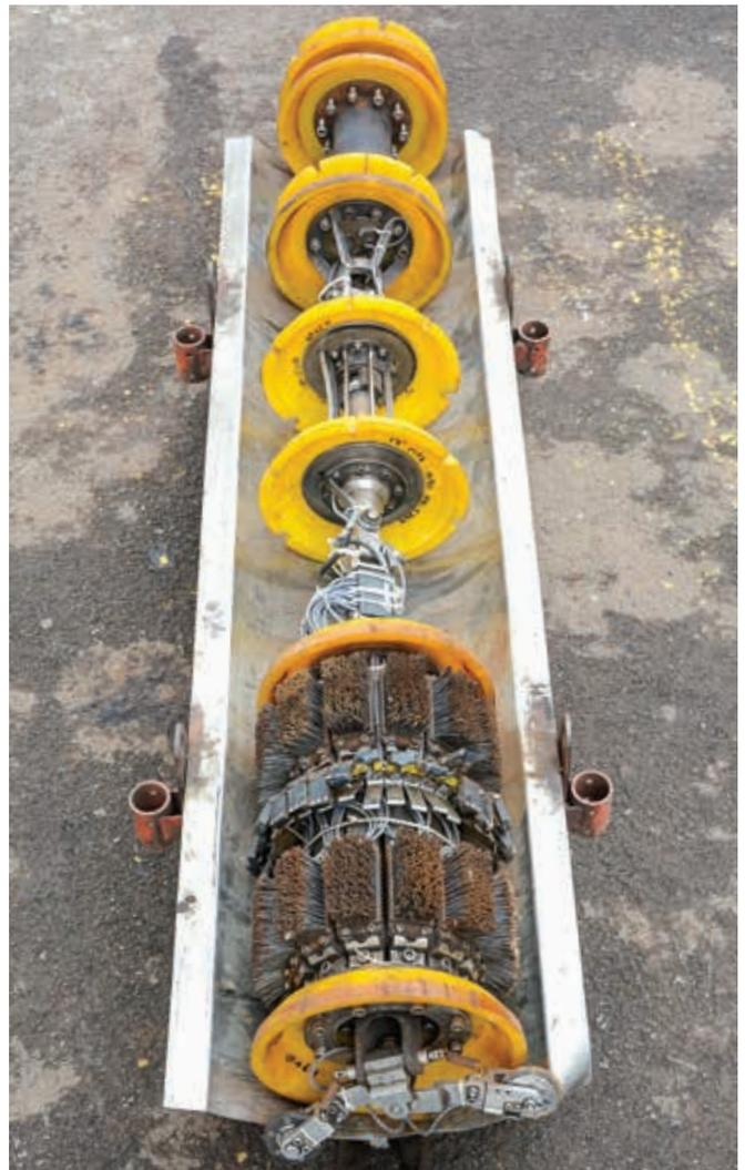
→ Pipeline Integrity check using Inspection Gauge
