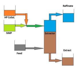
HPCL developed HP CoSoL process to improve the lube raffinate yield improvement in solvent extraction unit. HPCoSoL process was implemented at Mumbai refinery and having high selectivity towards poly cyclic aromatics removal. HP CoSoL process could be used for all grades of lube oil production.
