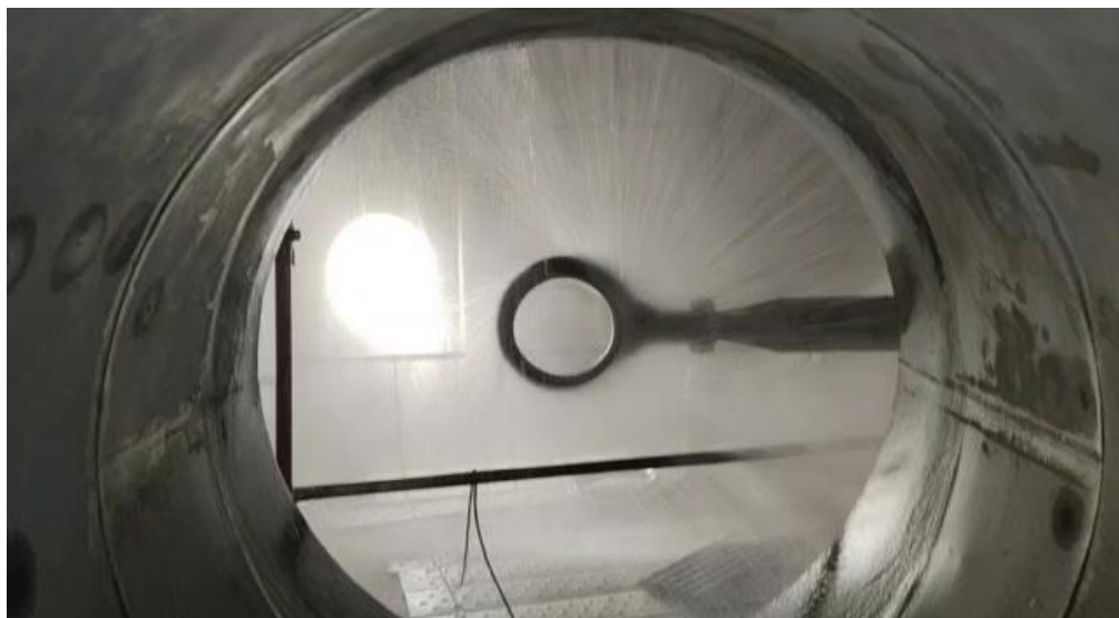
Spray Pattern of R&D supplied Scrubber Nozzle at MR
